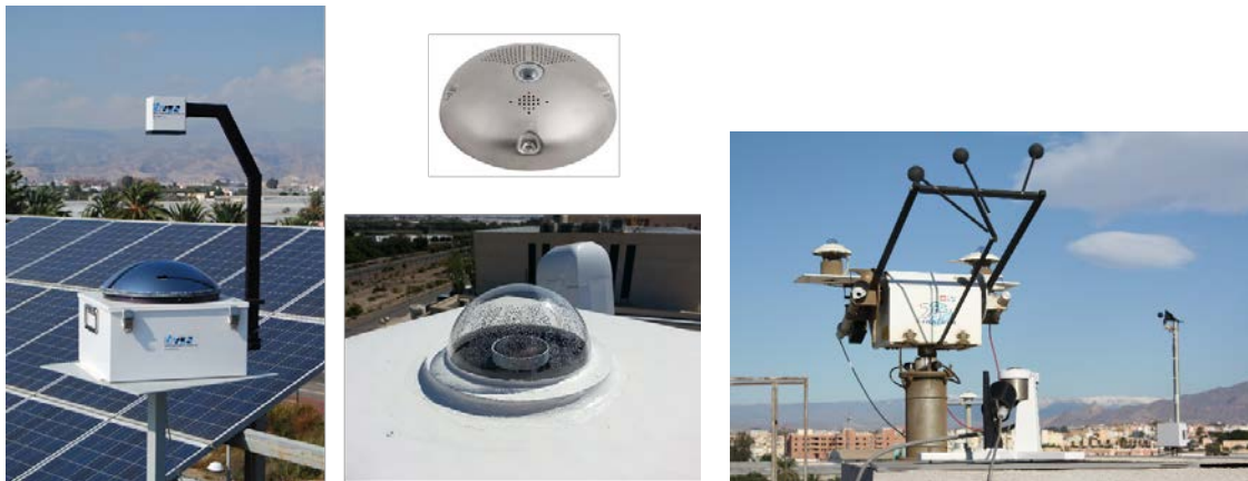
Cloud prediction system. Real-time cloud prediction up to 3 hours ahead, using satellite imagery and sky cameras.
