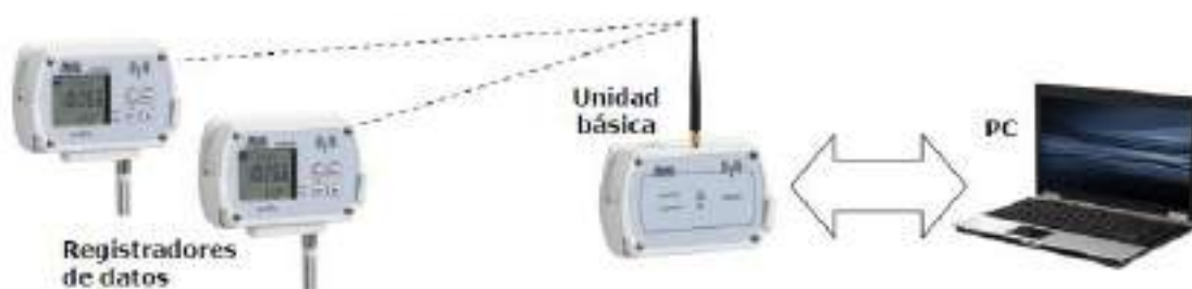
Generic schematic of base unit connected between data loggers and PCs
