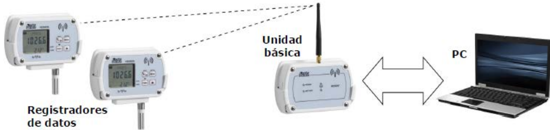
Generic schematic of base unit connected between data loggers and PCs
